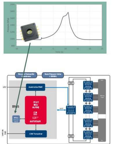
Two options for pressure increase detection with the absolute pressure sensor
