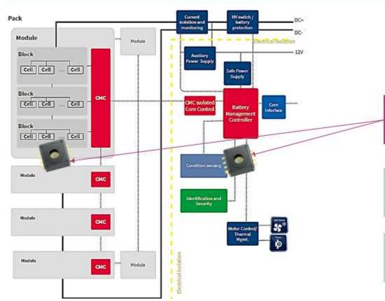
Barometric Pressure Sensor for Thermal Runaway detection can be placed inside battery pack housing or inside central control box (BMS)
