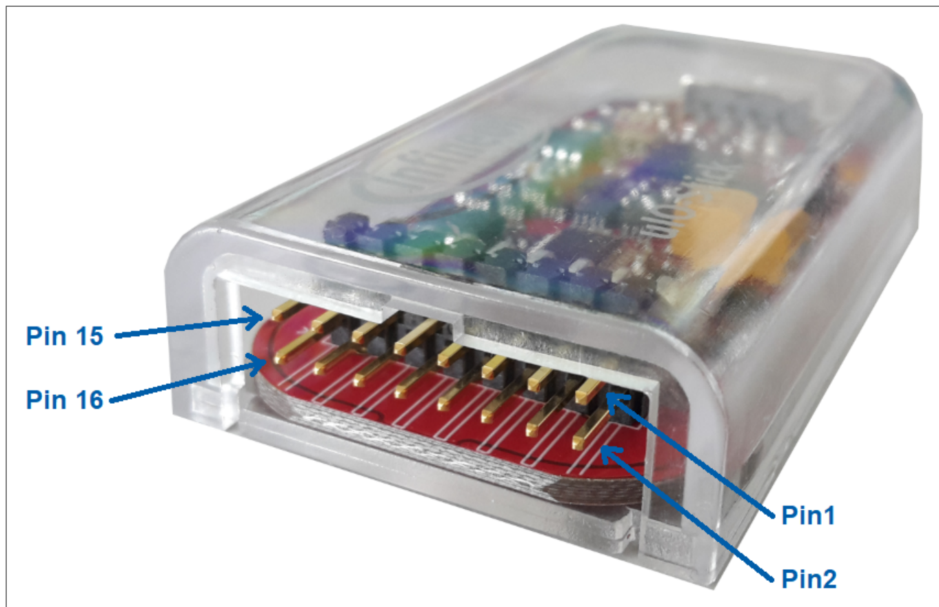
Figure 2 μIO-Stick pin view
