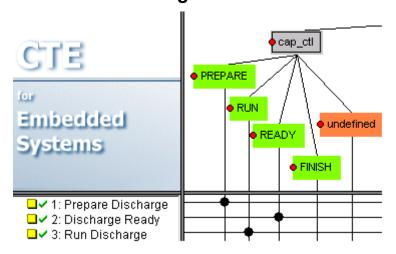
To determine the necessary test cases for each function, the Classification Tree Method was used. This allows an easy review of the testing ideas. Often, test data could be specified in the classification tree. For a function, typically 15 test cases were necessary, but some functions needed up to about 100 test cases. For each function the branch coverage (also known as
